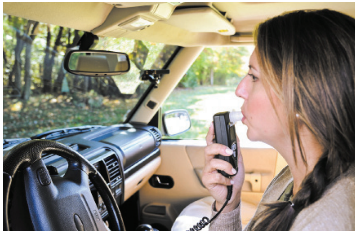
Ignition interlock devices will keep a car from going anywhere if a driver tests positive for alcohol. PHOTO COURTESY OF LIFESAFER
